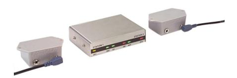
Oriteq-1600 is a versatile continuous monitor specifically designed for those price sensitive customers. It is base on a unique, accurate, low voltage, resistive loop detection technology. Being manufactured by precision SMT technology along with its compact stainless steel housing, it is able to sustain supreme reliability. Oriteq-1600 can monitor the groundings of 2 ESD wrist straps (35 M / 1.8 M), 2 ESD Mats (3.5 M), and 2 sets of low resistance (10 Ohm) machines.
