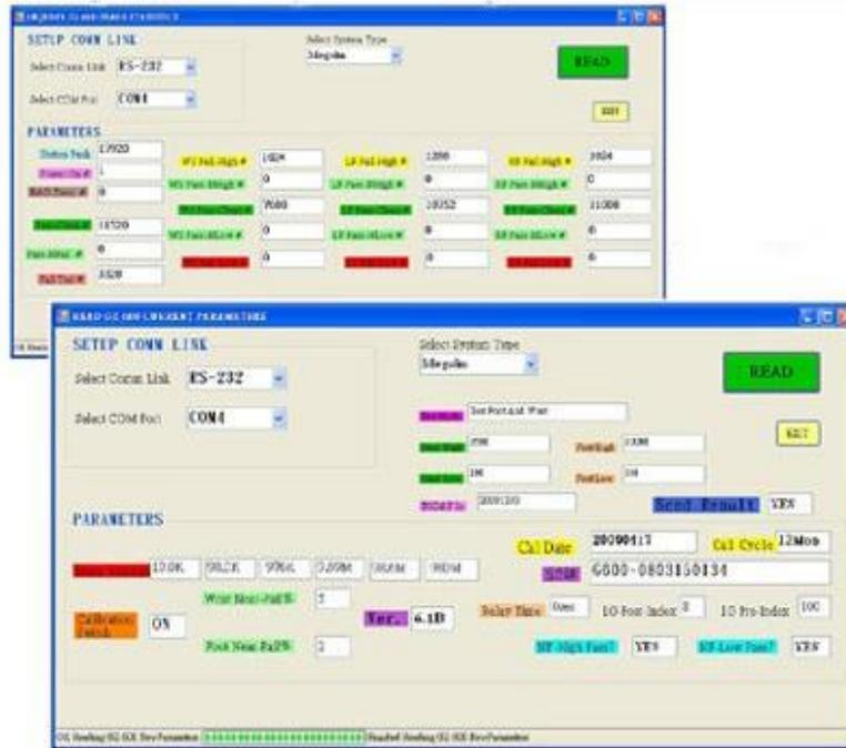
This stand-alone program designed for the hardware management of the Captain GREEN Series defensive ESD testers. It uses the RS-232 serial port to communicate with the tester hardware for data exchange. The main functions are to read the tester's internal control parameters and usage statistics and to set new control parameters.
