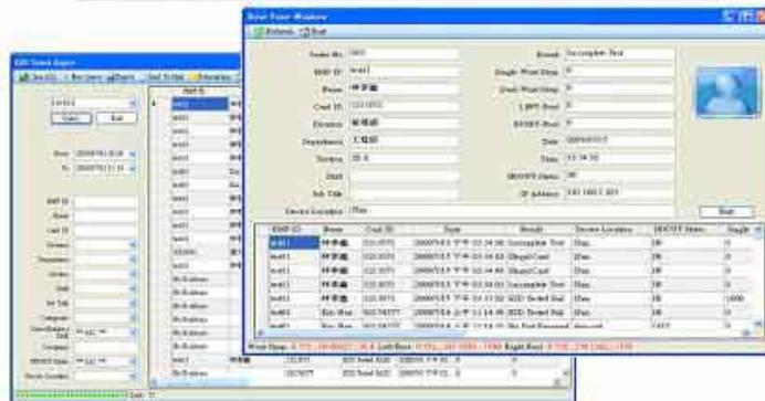
The integrated management software specifically designed for the GZ-600 / GZ-350 Captain GREEN Defensive testers. It provides the users easy-to-use and powerful functions including employee access administration and automatic statistical and analytical reports generation of test results. GZ-600-IMS can be used with a GZ-600 /GZ-350 in stand-alone or networked mode. It runs on a PC and connects to the GZ-600 / Oriteq-350 through the TCP/IP jacket in the Local Area Network (LAN).
