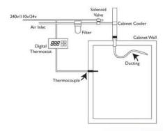
For example, if the cabinet overheats when its internal temperature reaches 32°C the digital thermostat can be set to turn the cabinet cooler on when the internal temperature reaches 29°C and off once it
