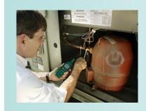
Compact meter is well-suited for field applications. Unique sensor cap closes for protection during storage. Simultaneously displays relative humidity, air temperature and dew point or wet bulb. Calculates T1-T2 differential (air temperature minus external probe temperature) using optional probe (TP890), and T2 minus dew point. Other features include Data Hold, Auto Power Off, and MAX/MIN
