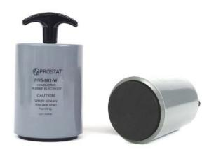
The PRS-801W is a precision milled resistance probe with conductive rubber pad for use with any resistance meter. Used in point to point and point to ground resistance testing of floors, worksurfaces, floor mats or any flat object, the PRS-801W produces repeatable measurements in accordance with ESD Association standards.
