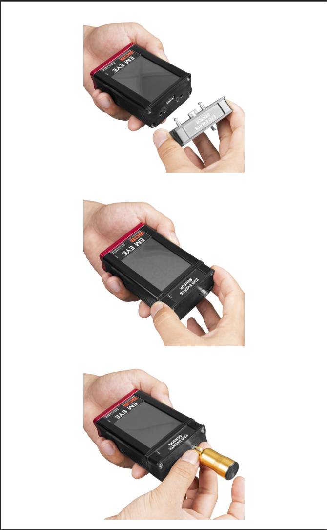
Figure 6. Attaching the sensor module to the EM Eye Meter
