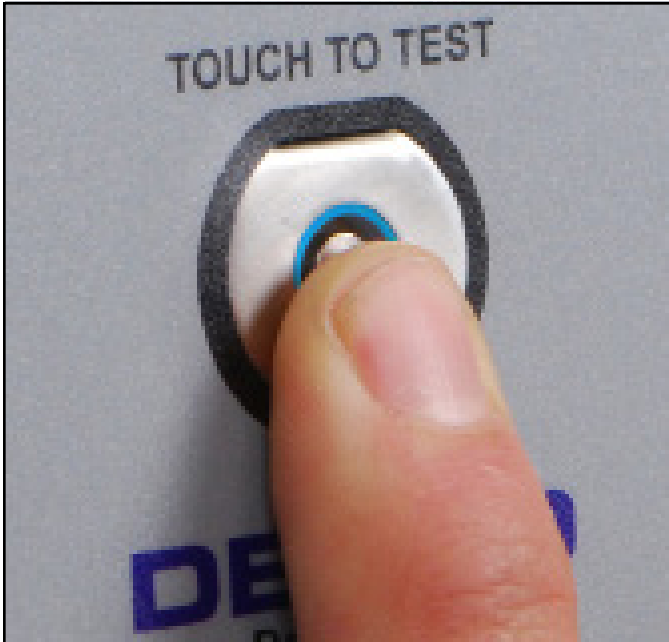
Figure 11. Bridging the test switch's contacts to initiate the test
