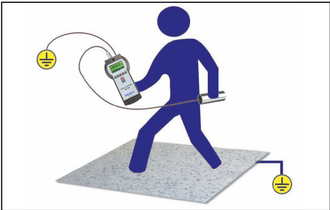
Figure 3. Setup of the Body Voltage Meter
