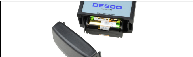
Figure 9. Replacing the batteries
