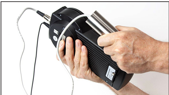
Figure 4. Touching the ground touch plate to ground the operator and zero the meter
