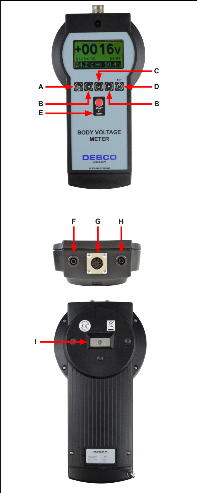
Figure 2. Body Voltage Meter features and components
