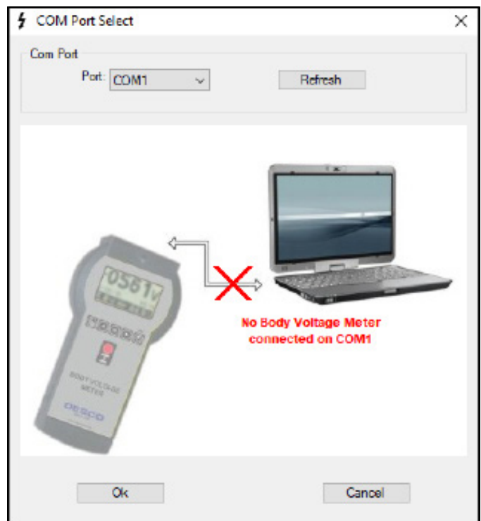
Figure 6. Selecting a COM port using the WT Manager software
