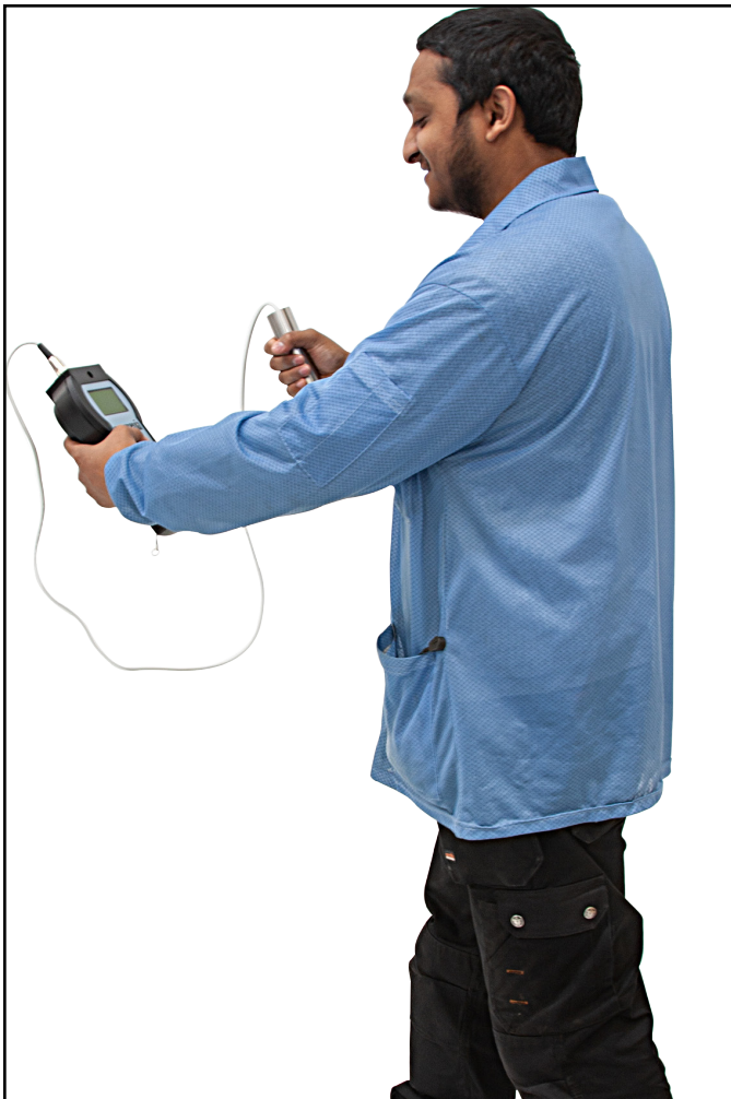
Figure 5. Using the Body Voltage Monitor
