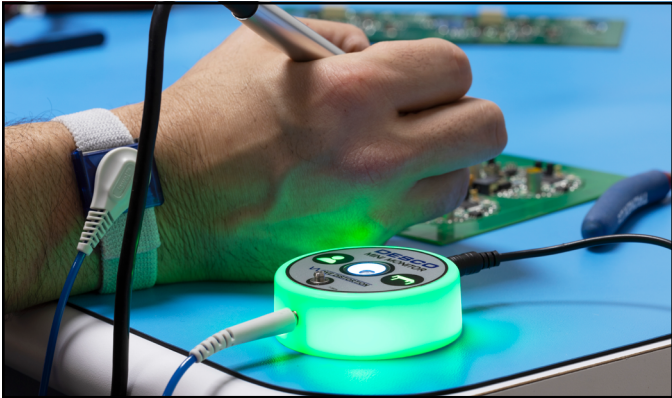
Figure 8. Illuminating green to indicate a proper operator path-to-ground
