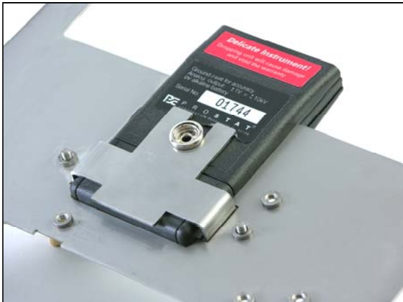
Figure 4: Seat the PFM-711A into Field Meter Saddle
