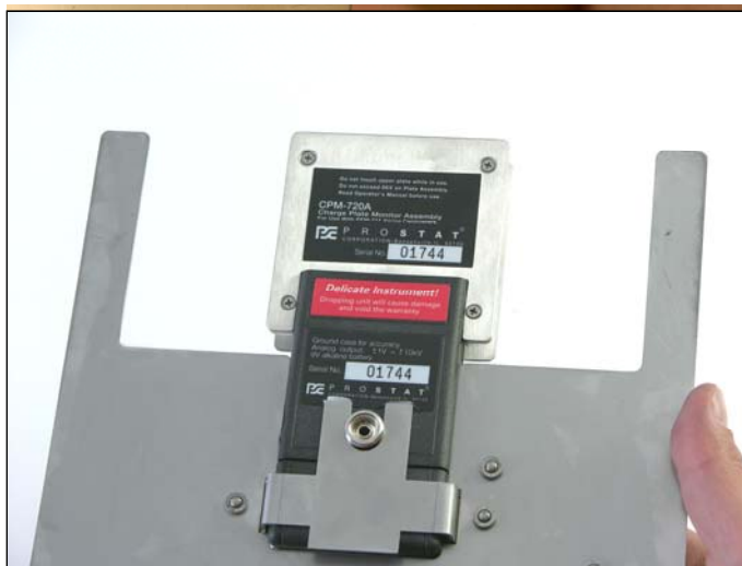
Figure 13: Field Meter fills the CPM-720 Lower Ground Plate to completely seat the plate assembly.
