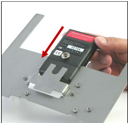
Figure 3: Mount PFM-711A into Carrier Plate
